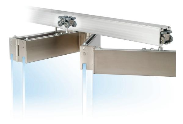
The SLF400 Slide and Fold Glass Panel System features a straight sliding aluminium top track. This system is able to carry frameless glass door panels of up to 2700mm high and width of up to 750mm.
